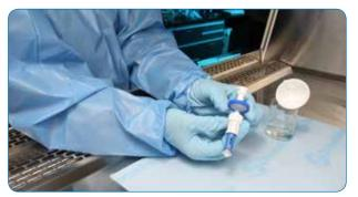
2 Engage this assembly onto Vial Assembly to create Filter Assembly.
