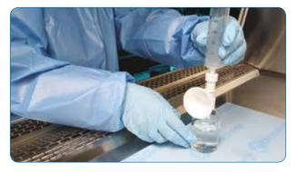
**3** Disengage Syringe Unit 1 from Vial Assembly.
