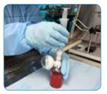
3 Invert system and aspirate drug dose into Syringe Unit. Expansion chamber will deflate.
