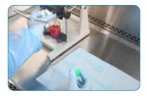
4 Using downward force on handle, attach Protector onto vial to create Vial Assembly.
